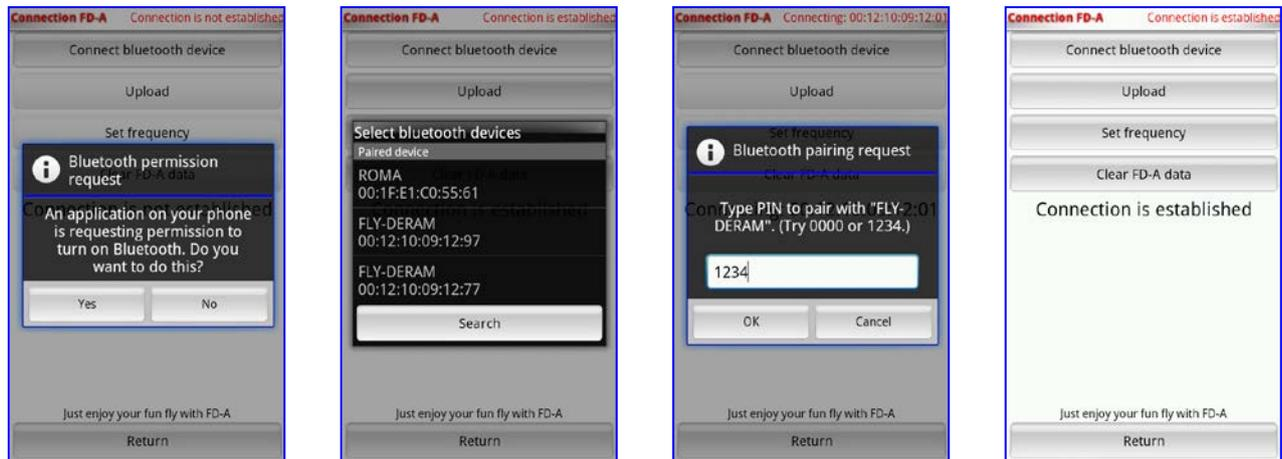
In setup interface, users can upload the data of FD-A altimeter, also can set up the frequency of FD-A and clear the data of FD-A.
